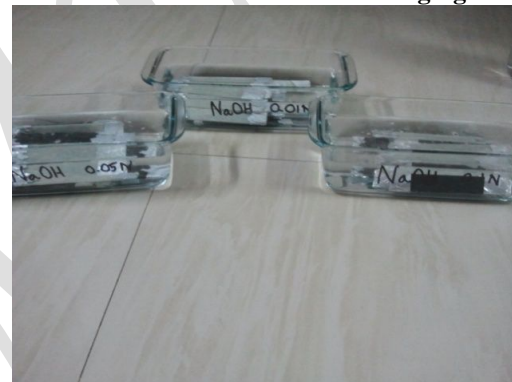
Figure 2b : specimens immersed in NaOH solution of different concentration for aging
