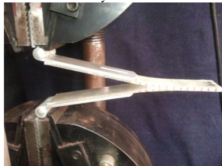
Figure 3a : crack propagation in glass-epoxy composite under DCB test
