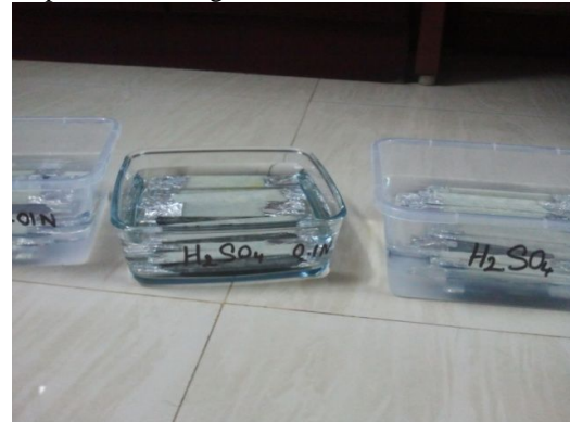
Figure 2a: specimens immersed in H 2 SO 4 solution of different concentration for aging
