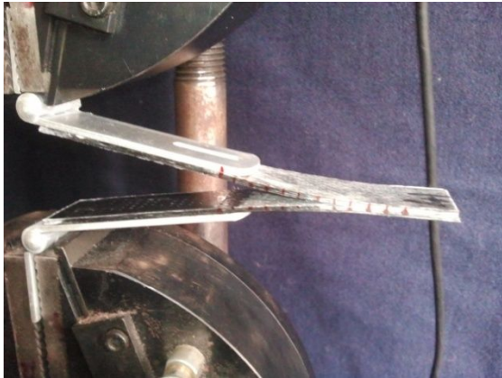
Figure 3b : crack propagation in glass-carbon hybrid composite under DCB test
